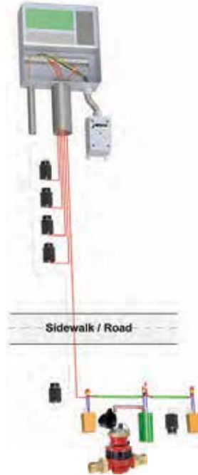
Adding 2-Wire, master valve and flow sensor using existing conventional wires
