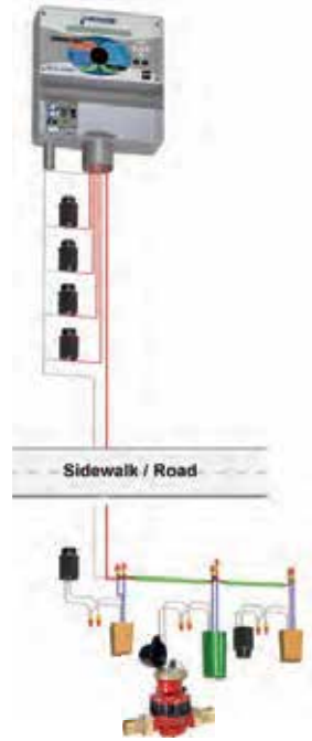
Adding 2-Wire, master valve and flow sensor using existing conventional wires
